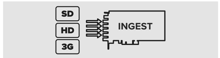
**4 simultaneous and independent streams** allows capture of multiple inputs from a range of 3G/HD/SD-SDI sources. Each channel can be capturing a different resolution, frame-rate, and/or codec.
